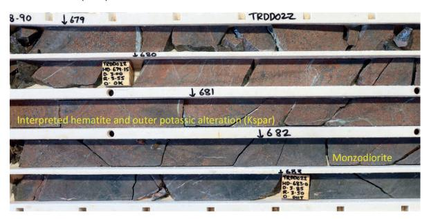
(b) Monzodiorite (light-grey) with strongly developed and variable red alteration (interpreted hematite and outer potassic) along with fine magnetite veinlets (black) and some quartz veins (white), from 679m down hole.
