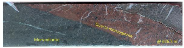
(a) Monzodiorite (grey) cut by orange-red quartz-monzodiorite at 626.5m down hole, in turn cut by quartz-carbonate veinlets (white).
