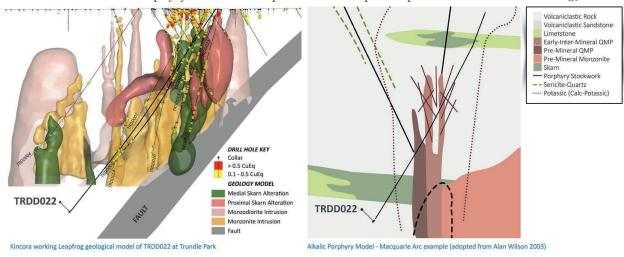
Below shallow skarn alteration, TRDDo22 intersected a thick interval of equi-crystaline monzodiorite from 376m to 723m depth, which was expected from the geological model (Figures 4, 5 and 6). Notable and positive indicators include:
