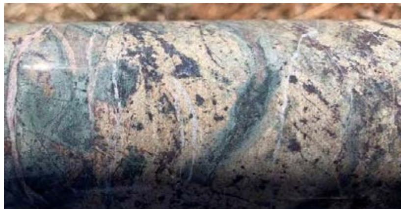
Qz-Ch-Ser altered skarn with patchy chalcopyrite and bornite: 2.44g/t gold & 0.20% copper @ 286-287m
