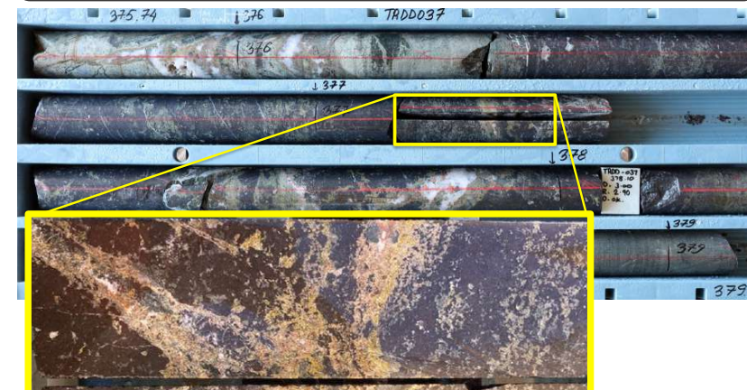
TRDD037: Massive magnetite skarn with minor patches of garnet (brown) and pyroxene (tan-green) @ 376.3-406.8m. Disseminated py -/+ cp. Minor patches of retrograde calcite & orthoclase fill voids & fractures*
