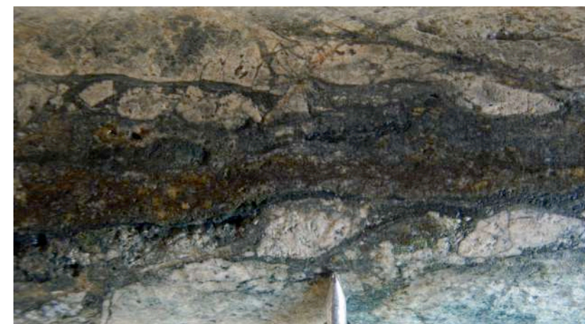
TRDD036: qtz-cp-py vein with overprint carbonate-ab-silica-hm-ab (within 0.5m @ 1.72g/t Au, 2.54% Cu & 721ppm Mo from 96.4m)
