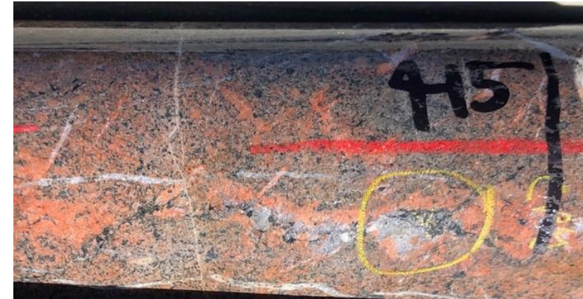
Altered quartz-monzodiorite with quartz-pyr-cp veining and vein selvage potassic alteration @ 415m
