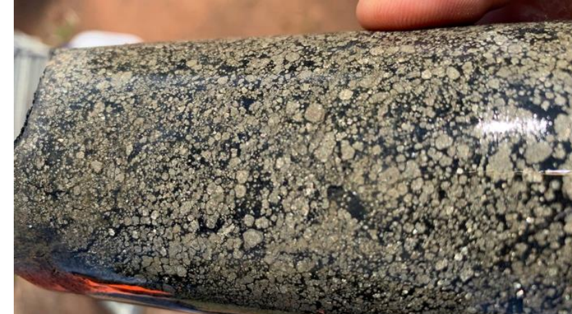
Coarse pyrite in skarn: 0.63g/t gold & 3.4% copper @ 64.1-65m
