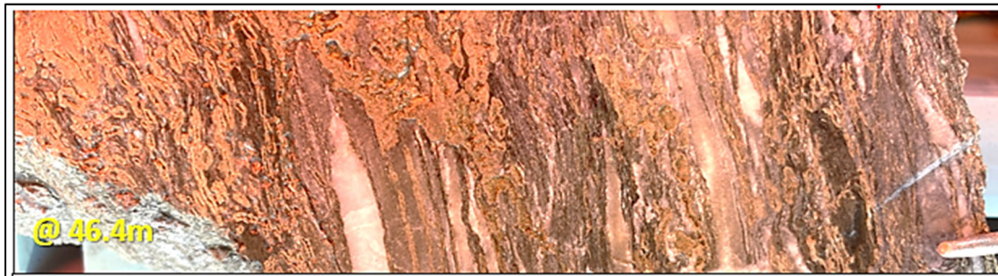
Photo 1: Deformed and foliated phyllite (grey) with quartz veins (white) cut by pyrite-arsenopyrite (yellow-tan) veining along the foliation in hole CDDH001 at 46.4m down hole Occurs in the interval containing 1m at 9 g/t gold and 530 g/t silver from 46m
