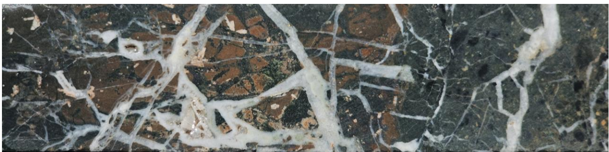
Hole NEDD005 - 358.6m: stockwork chalcopyrite-pyrite bearing quartz-carbonate veins intersect silicified, brecciated dacite porphyry, returning elevated copper (235 ppm) with minor molybdenum and zinc.
