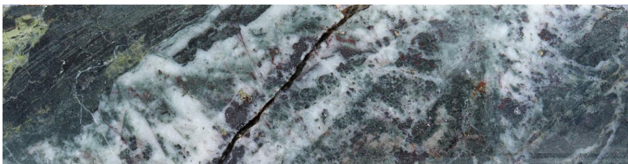
Hole NEDD007 - 384.45m: chalcopyrite-pyrite-bornite rich quartz-carbonate-specular hematite veining intersecting weakly propylitically altered intermediate volcanic rocks, returning elevated copper (3400 ppm) and gold (0.341 g/t), with minor molybdenum, silver and zinc
