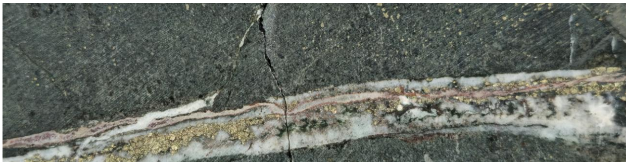
Hole NEDD006 - 417.25m: chalcopyrite-pyrite bearing quartz-carbonate-chlorite-hematite vein and disseminated chalcopyrite-pyrite within weakly propylitically altered intermediate volcanic rocks with elevated copper (234 ppm) with minor gold, molybdenum, silver and zinc
