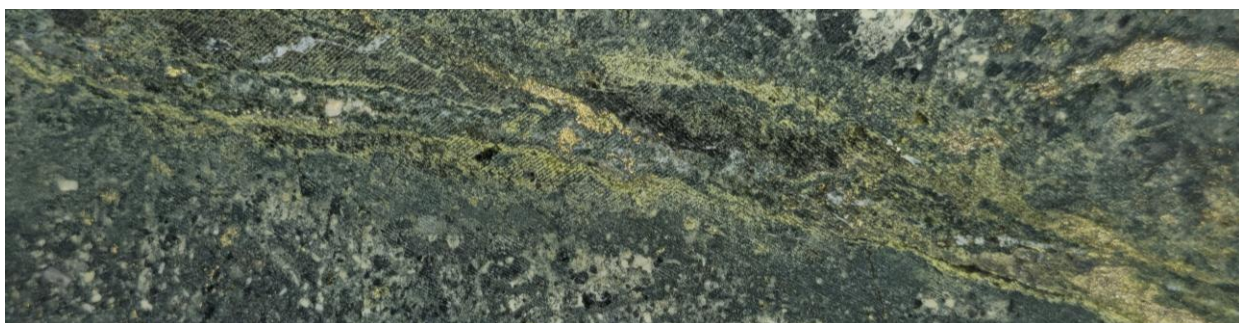
Hole NEDD007 - 519.5m: chalcopyrite-pyrite rich quartz-carbonate-chlorite veins intersecting strongly propylitic-sodic altered hydrothermal breccia, returning elevated copper (13700 ppm) with gold (0.475 g/t) and molybdenum (31.8 ppm) with minor silver, lead and zinc.
