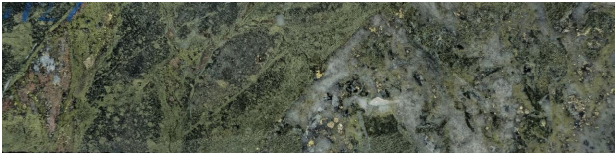
Hole NEDD006 - 337.15m: chalcopyrite-pyrite bearing quartz-carbonate veins cutting strongly propylitic altered intermediate volcanic rocks, returning elevated copper (4470 ppm) with minor gold, molybdenum, silver and zinc.
