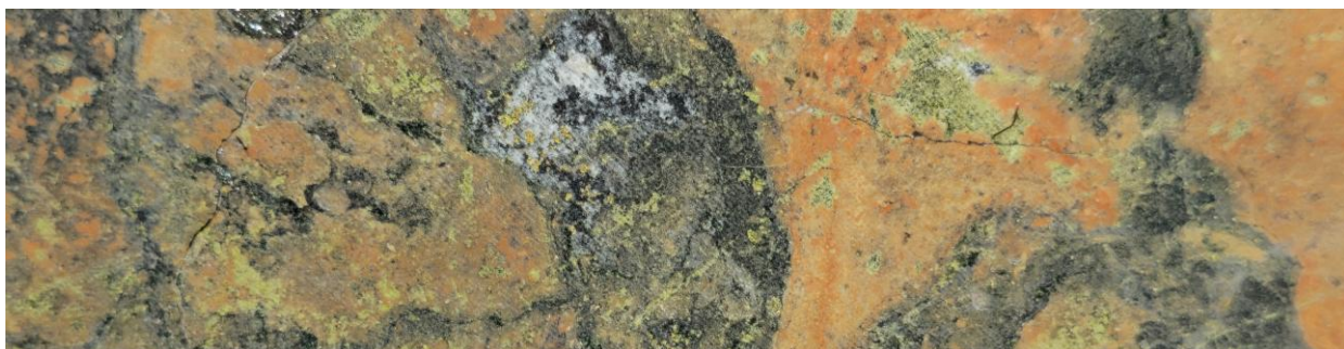
Hole NEDD007 - 557.4m: hydrothermal breccia with a quartz-carbonate+chlorite cement hosting disseminated chalcopyrite mineralization, returning elevated copper (812 ppm) and gold (0.28 g/t) with minor molybdenum and silver
