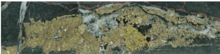
Hole NEDD006 - 407.7m: chalcopyrite-pyrite rich quartz-carbonate-magnetite-hematite veins intersecting weakly propylitically altered intermediate volcanic rocks, returning elevated copper (1310 ppm) with gold (0.431 g/t) and minor molybdenum, silver and zinc.
